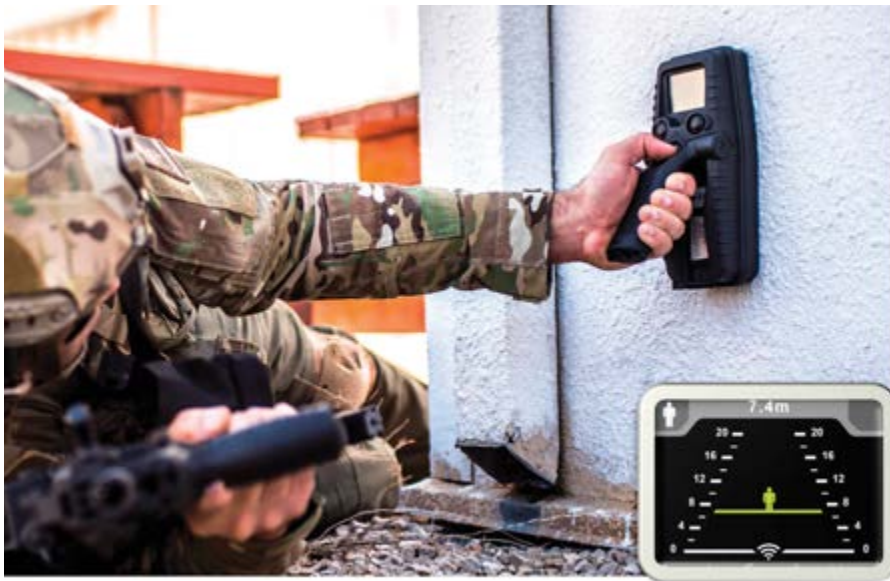
The Xaver 100 encompasses Camero's See-Through Technology at the lowest tactical level, and provides assault teams with situation awareness before breaching.
