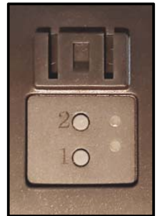
Transceiver Base Station's Programming Pad (Clip Removed)
