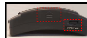
Transceiver Base Station Battery Compartment & "POWER ON/OFF VOL." Dial
