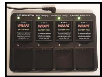
Battery Packs Inserted into Battery Charge Station Bays
