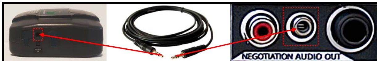
Transceiver Base Station Connected to External Audio Source's 1/8" (3.5mm) Audio Out Jack via 25 ft. Audio Cable
