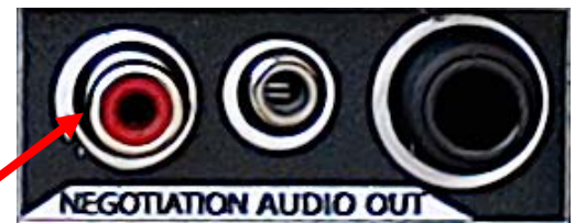
Direct-Link Bridge Series System "NEGOTIATION AUDIO" RCA output jack (located on outer/right of Command Console)
