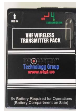
VHF Wireless Transmitter Pack (includes 9v Non-Rechargeable Battery)
